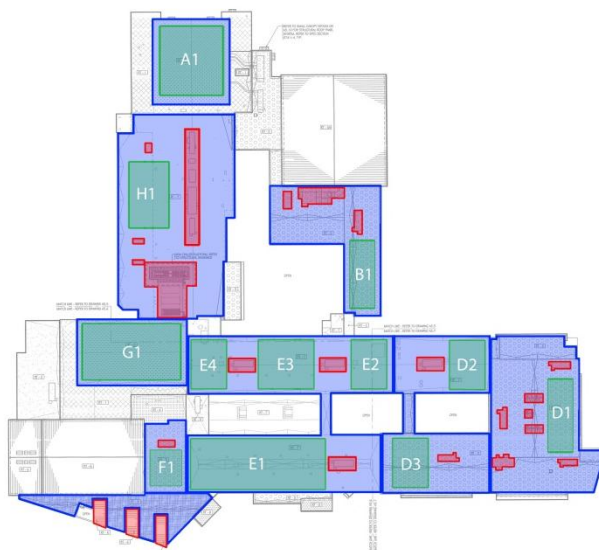
Figure 25: Roofs Selected for PV Array Installation
