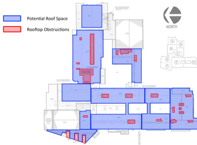
Figure 24: Potential Roof Space
